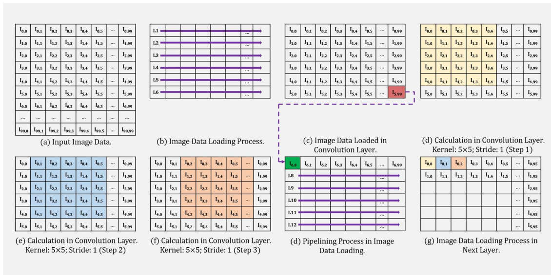
Fig. 2. Pipelining architecture of the proposed HePiLUT CNN accelerator.
